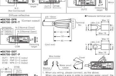
wire should be \$6-10mm and tighten wire holder with 1.0 t
