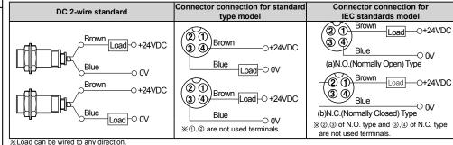
No need to consider polarity for non-polarity type of power supply.
