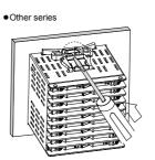
\* Insert product into a panel, fasten bracket by pushing with tools as shown above
